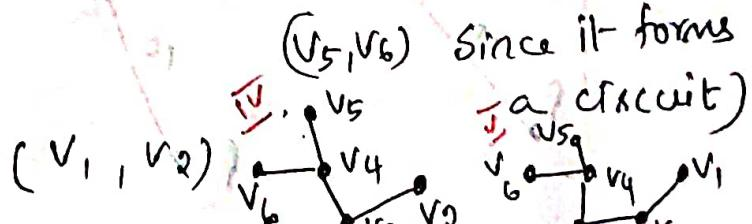
5 edges of smallest weights have been selected and the minimal spanning tree is
