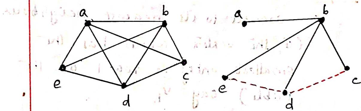
Adding the chord  $(c,d)$  to the spanning tree  $T$  will form a fundamental circuit  $bcdcb$ .
